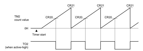
Figure 11-50. Example of Timer/Event Counter 2 PPG Signal Output
