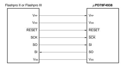
Figure 28-4. Flashpro II and Flashpro III Connection in UART Mode
