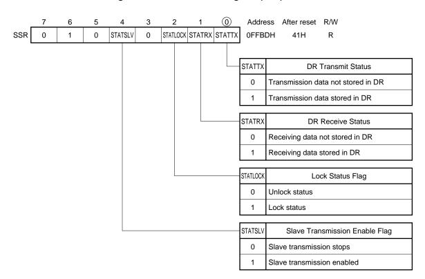
Figure 20-25. Slave Status Register (SSR) Format
