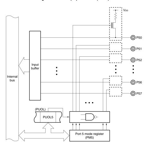
Figure 6-49. Pull-Up Specification (Port 5)
