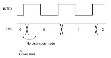
Figure 9-12. To Distinguish whether One or No Valid Edge has been Input with External Event Counter
