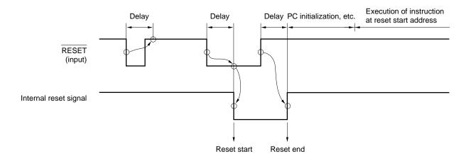
Figure 26-1. Reset Signal Acknowledgment
