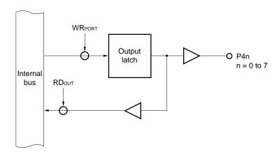
Figure 6-39. Port Specified as Output Port
