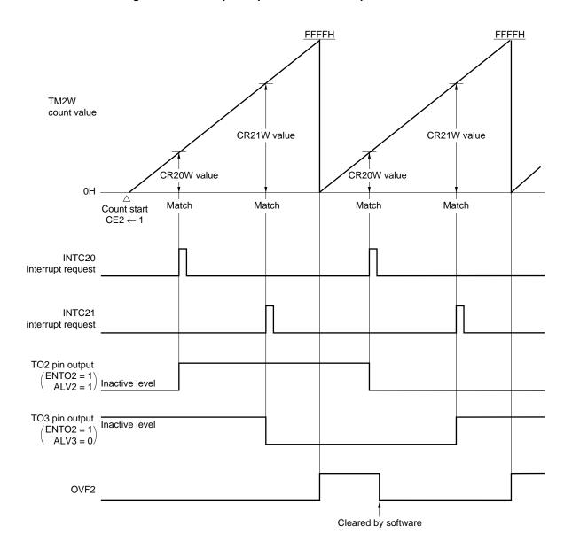
Figure 11-16. Compare Operation in 16-Bit Operation Mode
