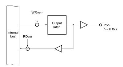
Figure 6-46. Port Specified as Output Port
