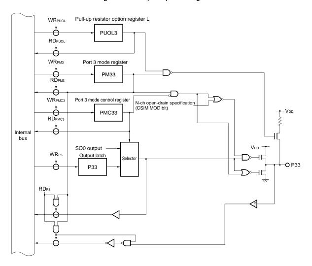
Figure 6-29. P33 (Port 3) Block Diagram
