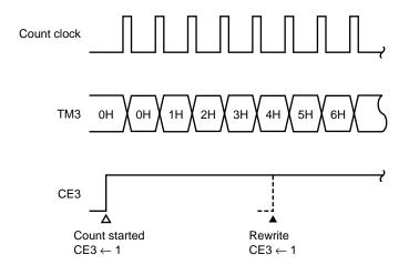
Figure 12-5. Basic Operation in 16-Bit Operation Mode (BW3 = 1)
