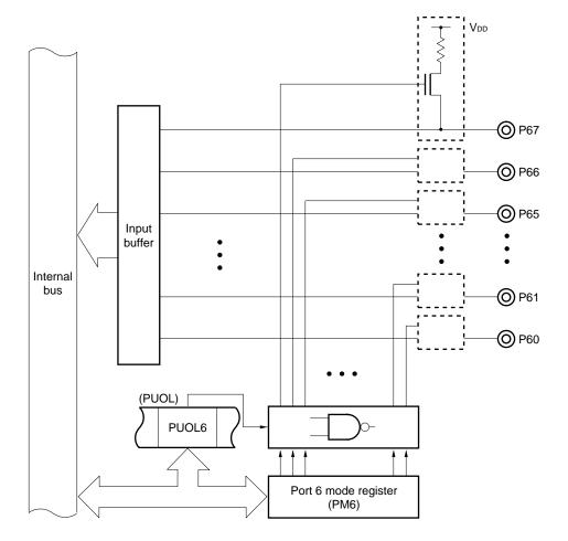
Figure 6-59. Pull-Up Specification (Port 6)
