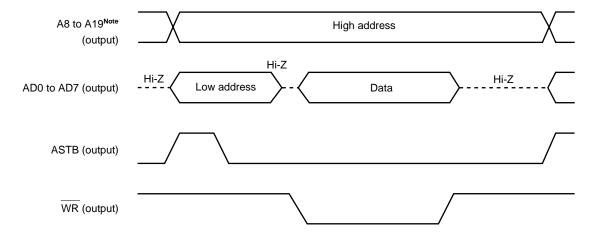
Figure 24-7. Write Timing
