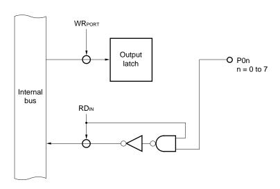
Figure 6-5. Port Specified as Input Port
