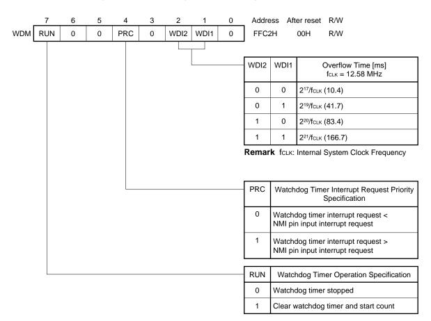
Figure 13-2. Watchdog Timer Mode Register (WDM) Format
