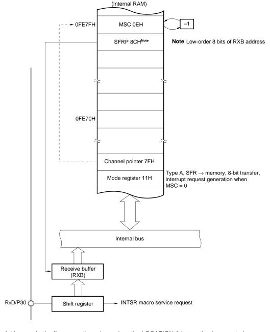
Figure 23-24. Asynchronous Serial Reception
