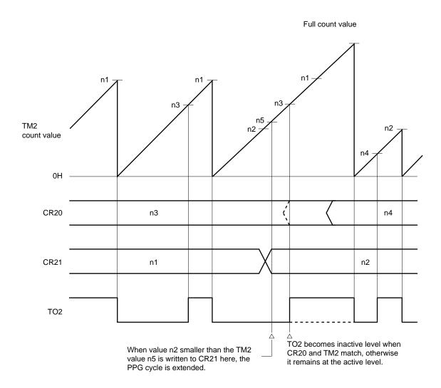
Figure 11-33. Example of Extended PPG Output Cycle
