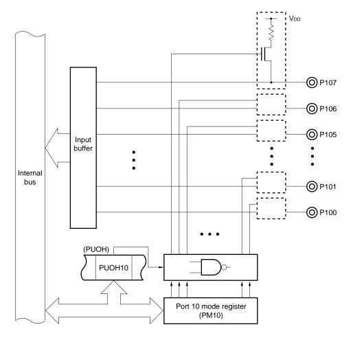
Figure 6-80. Pull-Up Specification (Port 10)
