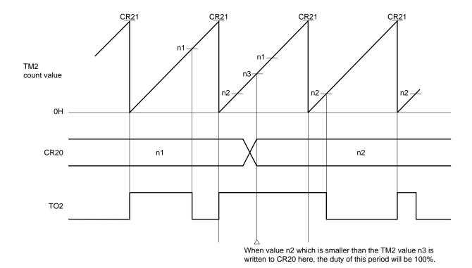
Figure 11-32. Example of 100% Duty with PPG Output
