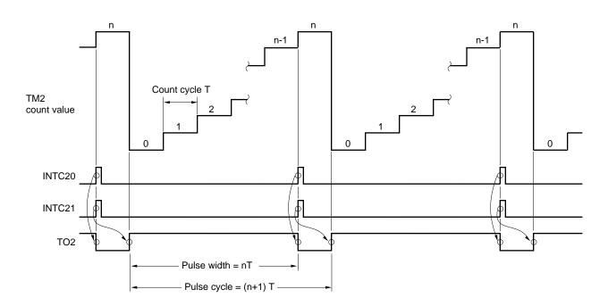
Figure 11-30. Example of PPG Output when CR20 = CR21
