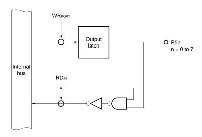
Figure 6-47. Port Specified as Input Port
