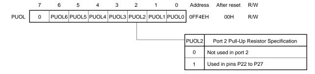
Remark When STOP mode is entered, setting PUOL to 00H is effective for reducing the current consumption.
