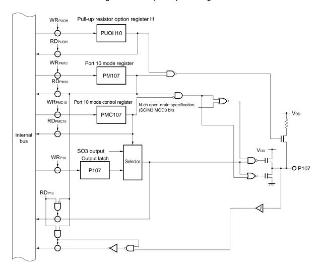
Figure 6-73. P107 (Port 10) Block Diagram
