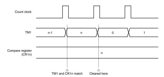
Figure 10-7. TM1 Clearance by Match with Compare Register (CR10, CR11)
