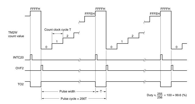
Figure 11-25. Example of PWM Output when CR20W = FFFFH
