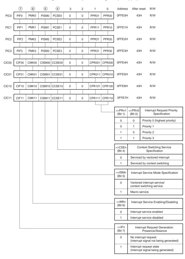
Figure 23-1. Interrupt Control Registers (××ICn) (1/4)
