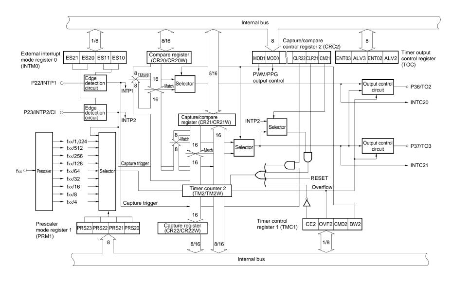
Figure 11-1. Timer/Event Counter 2 Block Diagram
