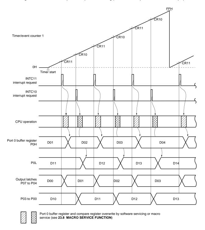
Figure 7-5. Real-Time Output Port Operation Timing (2-channel independent control example)
