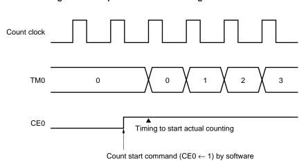
Figure 9-52. Operation when Counting is Started
