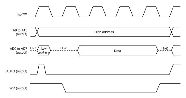
Figure 24-14. Timing with External Wait Signal
