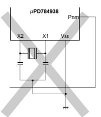
(d) Current flowing through ground line of oscillator
