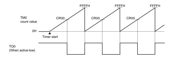
Figure 9-42. Control Register Settings for PWM Output Operation
