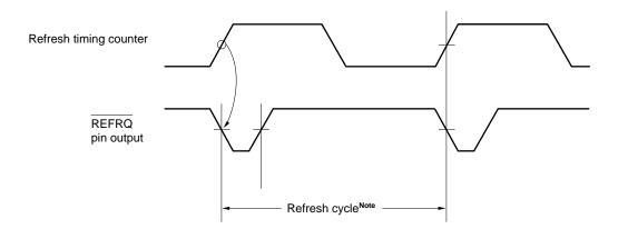
Figure 24-17. Pulse Refresh Operation in Internal Memory Access
