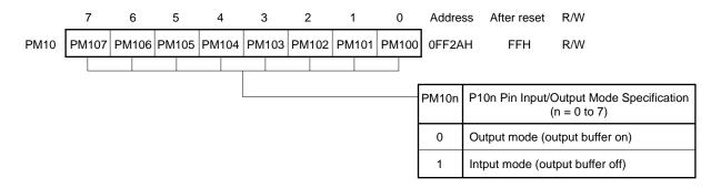
Figure 6-75. Port 10 Mode Control Register (PMC10) Format
