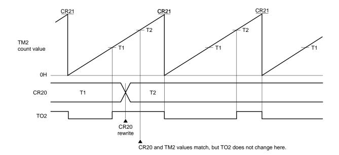
Figure 11-31. Example of Compare Register Rewrite
