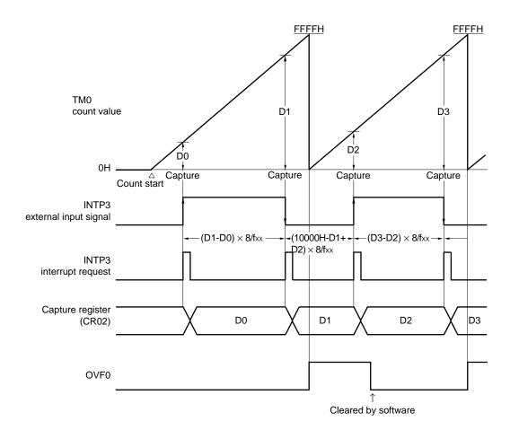
Figure 9-37. Pulse Width Measurement Timing
