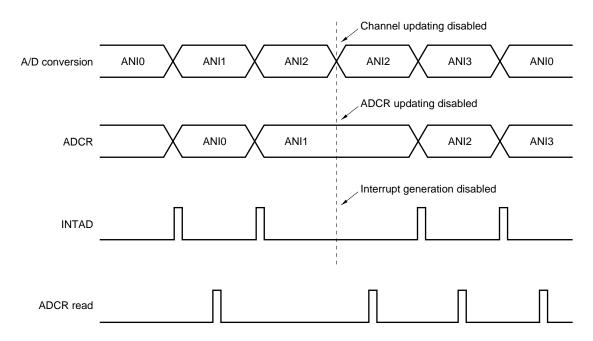
Figure 16-10. Scan Mode 1 Operation Timing
