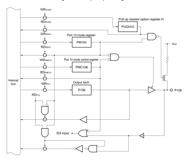
Figure 6-72. P106 (Port 10) Block Diagram
