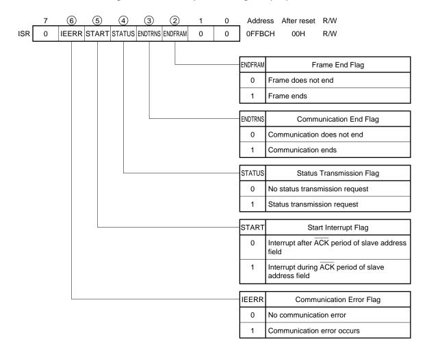
Figure 20-24. Interrupt Status Register (ISR) Format
