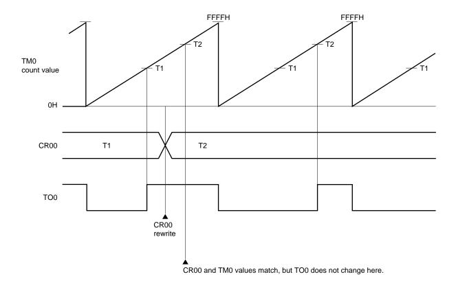
Figure 9-20. Example of Compare Register (CR00) Rewrite
