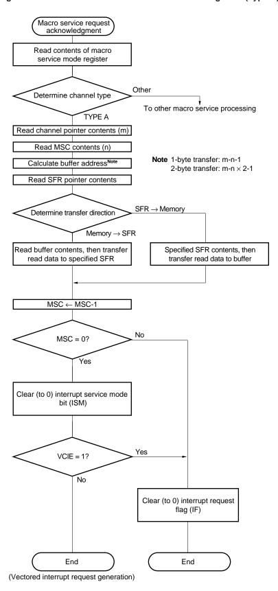
Figure 23-22. Macro Service Data Transfer Processing Flow (Type A)
