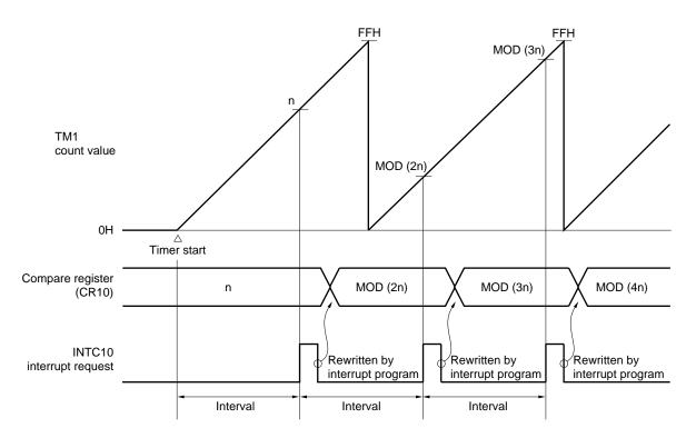
Figure 10-19. Interval Timer Operation (1) Timing
