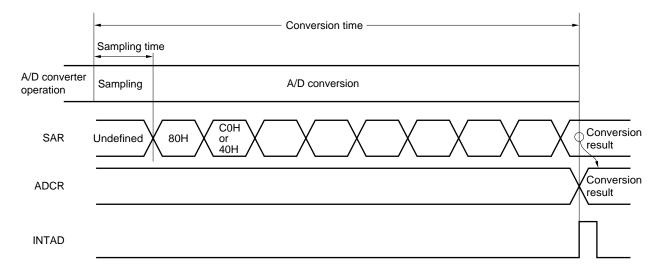
Figure 16-6. Basic A/D Converter Operation
