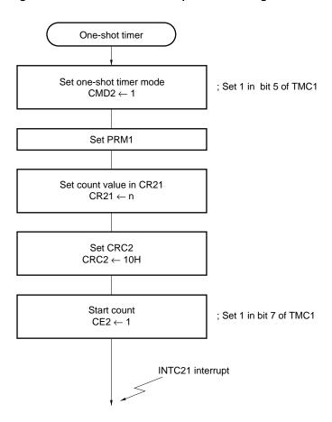
Figure 11-59. One-Shot Timer Operation Setting Procedure
