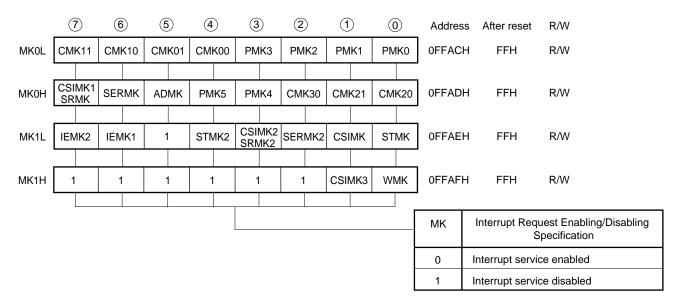
Figure 23-2. Interrupt Mask Register (MK0, MK1) Format (2/2)
