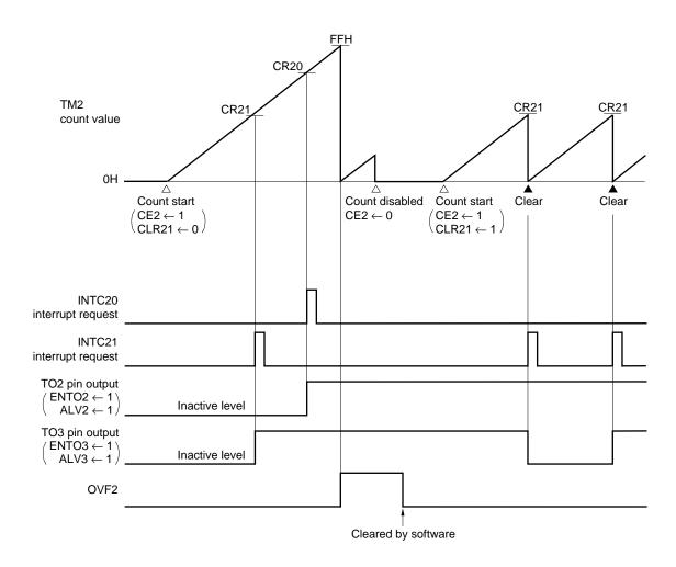
Figure 11-17. TM2 Clearance after Match Detection
