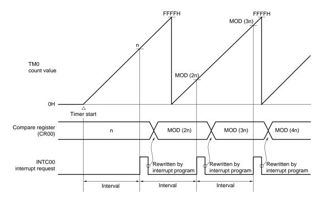
Figure 9-30. Interval Timer Operation (1) Timing
