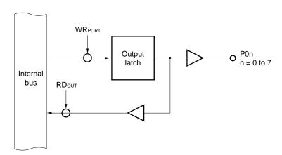
Figure 6-4. Port Specified as Output Port
