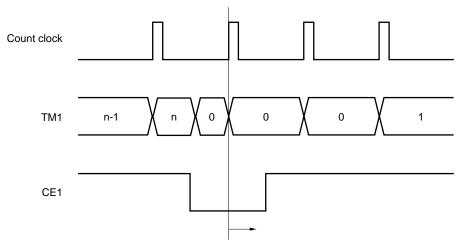
If the CE1 bit is set (to 1) from this count clock onward, the count clock starts counting from 0 after the CE1 bit is set (to 1).
