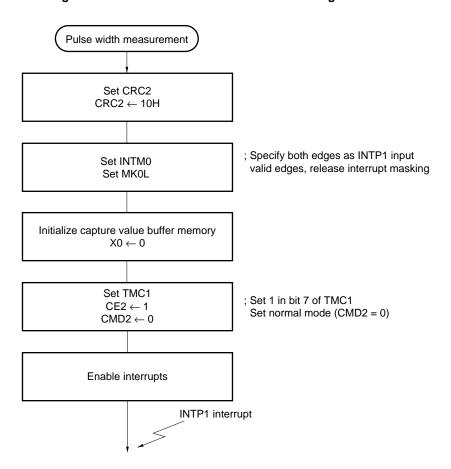
Figure 11-44. Pulse Width Measurement Setting Procedure
