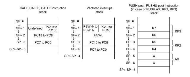
Figure 3-11. Data Restored from Stack Area
