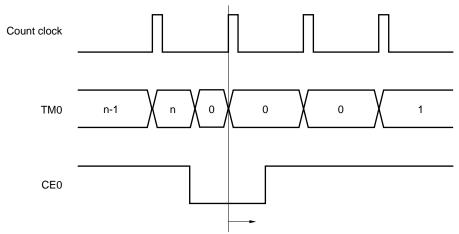
If the CE0 bit is set (to 1) from this count clock onward, the count starts from 0 on the count clock after the CE0 bit is set (to 1).
