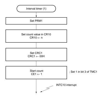
Figure 10-22. Interval Timer Operation (1) Interrupt Request Servicing
