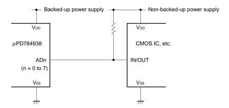
Figure 25-7. Example of Address/Data Bus Processing
