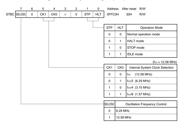
Figure 25-3. Standby Control Register (STBC) Format
