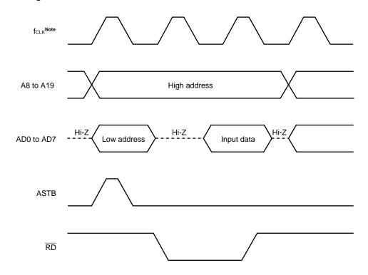
Figure 24-10. Address Wait Function Read/Write Timing (2/3)
