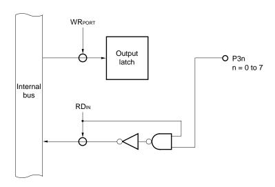
Figure 6-33. Port Specified as Input Port
