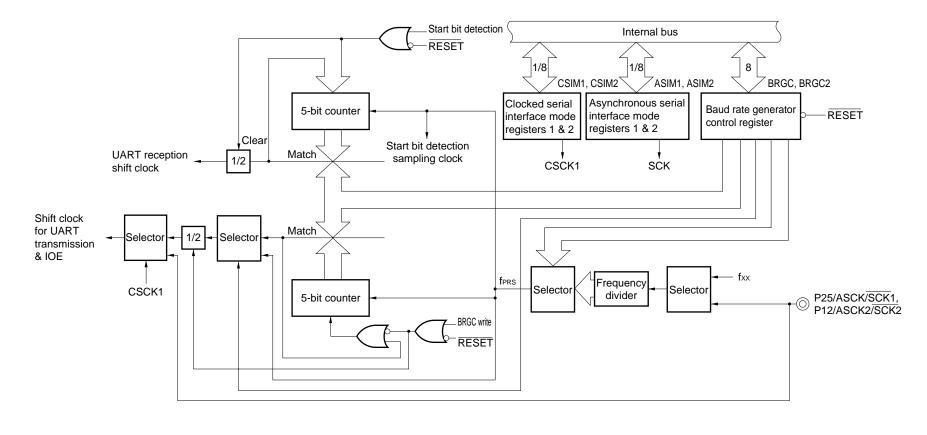
Figure 18-14. Baud Rate Generator Block Diagram
