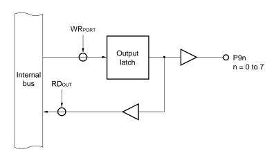
Figure 6-66. Port Specified as Output Port
