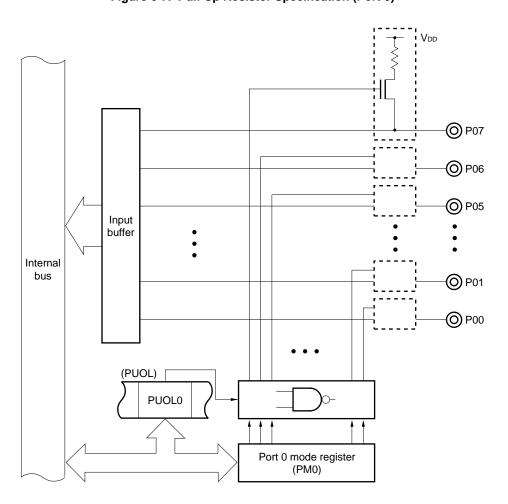
Figure 6-7. Pull-Up Resistor Specification (Port 0)
