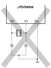
(c) Wiring near high fluctuating current
