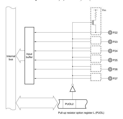
Figure 6-25. Pull-Up Specification (Port 2)
