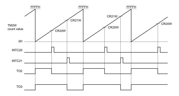
Figure 11-24. Example of PWM Output Using TM2W
