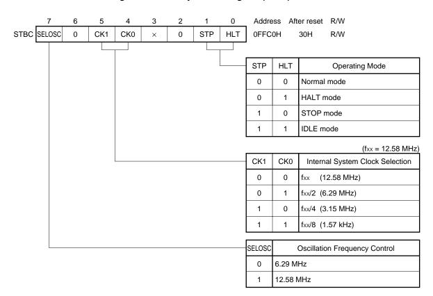
Figure 4-3. Standby Control Register (STBC) Format
