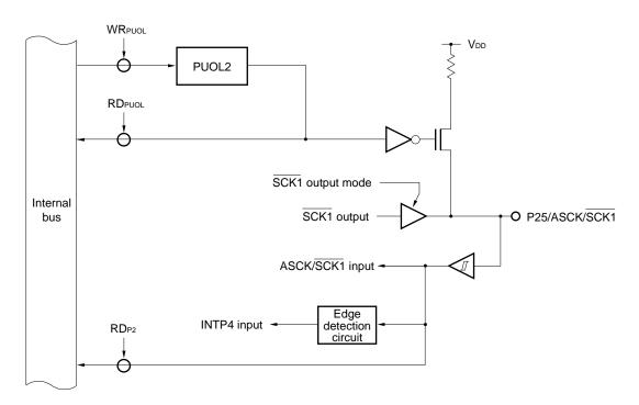
Figure 6-22. P25 (Port 2) Block Diagram
