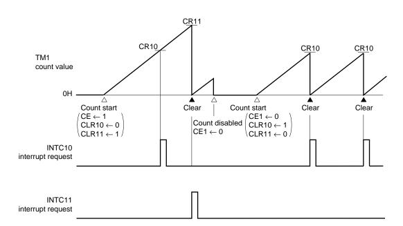
Figure 10-15. TM1 Clearance after Match Detection
