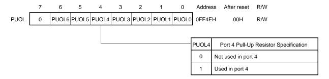
Caution When using the port 4 of the  $\mu$ PD784938 as an address/data bus pin, be sure to clear PUOL4 to 0 to disconnect the on-chip pull-up resistor.
