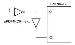
(3) The wiring connecting the X1 pin to the X2 pin via an inverter, in particular, should be made as short as possible.
