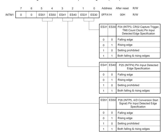
Figure 22-2. External Interrupt Mode Register 1 (INTM1) Format
