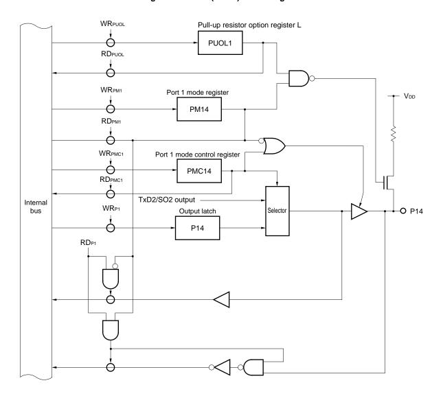
Figure 6-11. P14 (Port 1) Block Diagram
