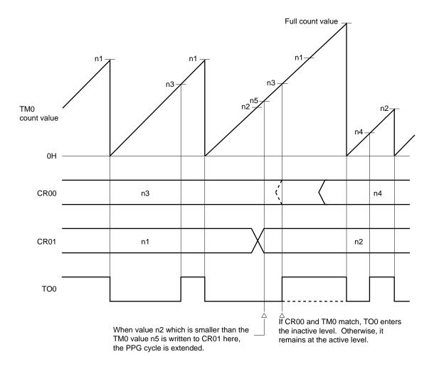
Figure 9-27. Example of Extended PPG Output Cycle
