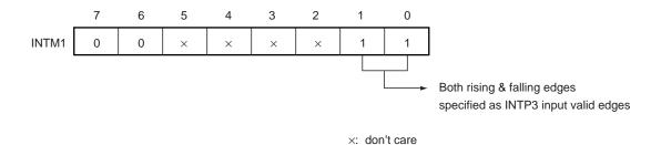
Figure 9-39. Pulse Width Measurement Setting Procedure
