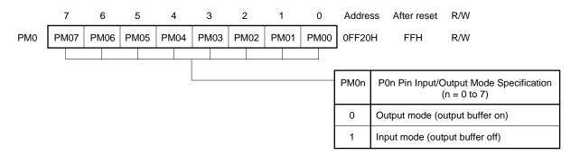
When port 0 is used as a real-time output port, the P0LM and P0HM bits of the real-time output port control register (RTPC) should be set (to 1).
