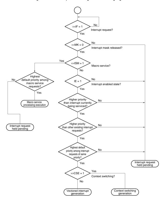
Figure 23-10. Interrupt Acknowledgment Processing Algorithm
