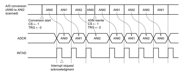
Figure 16-12. Software Start Scan Mode A/D Conversion Operation
