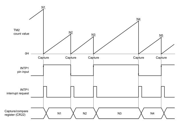
Figure 11-20. TM2 Clearance after Capture Operation
