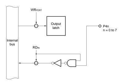
Figure 6-40. Port Specified as Input Port
