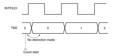
Figure 11-13. To Distinguish whether One or No Valid Edge has been Input with External Event Counter
