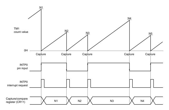
Figure 10-18. TM1 Clearance after Capture Operation
