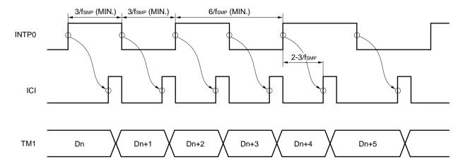
Remarks 1. ICI: INTP0 input signal after passing through edge detection circuit
