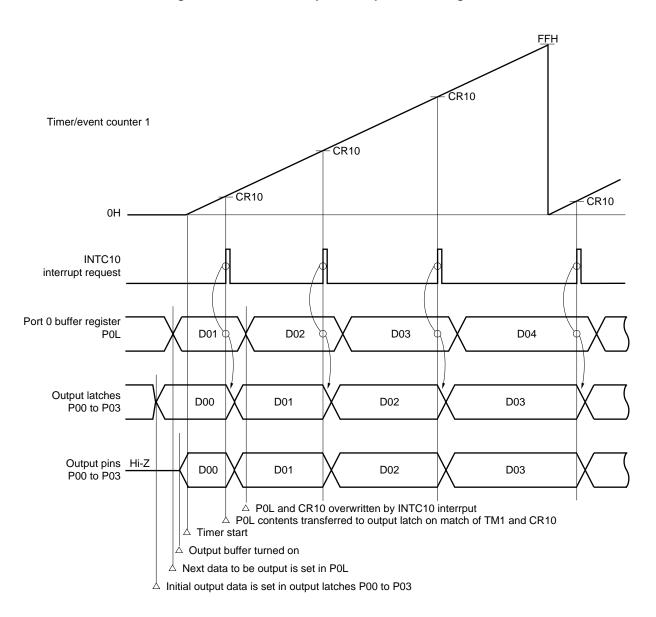
Figure 7-6. Real-Time Output Port Operation Timing
