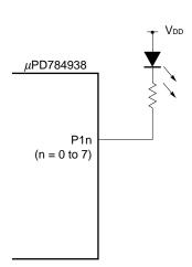
Figure 6-20. Example of Direct LED Drive
