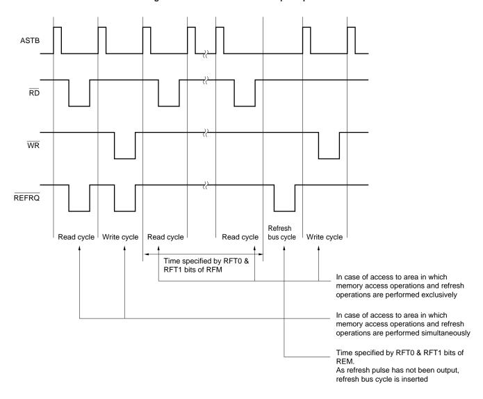
Figure 24-18. Refresh Pulse Output Operation
