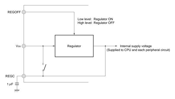
Figure 5-1. Regulator Peripherals Block Diagram
