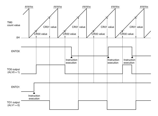
Figure 9-16. Toggle Output Operation
