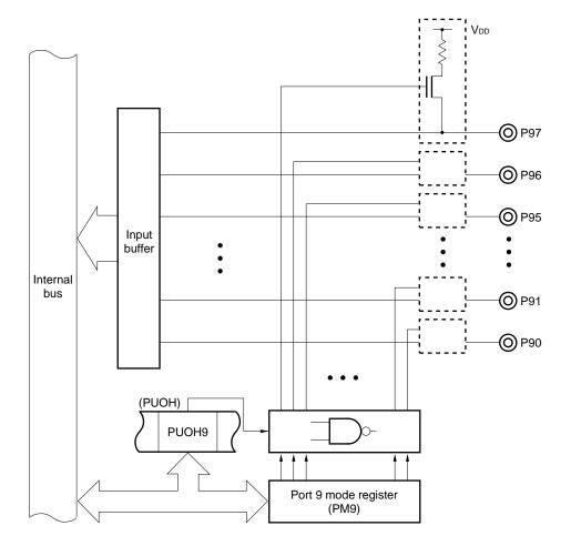
Figure 6-69. Pull-Up Specification (Port 9)
