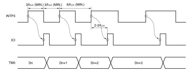
Remark ICI: INTP3 input signal after passing through edge detection circuit
