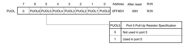
Caution When using the port 5 of the  $\mu$ PD784938 as an address bus, be sure to clear PUOL5 to 0 to disconnect the on-chip pull-up resistor.
