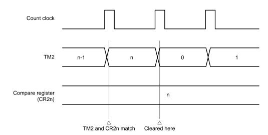
Figure 11-8. TM2 Clearance by Match with Compare Register (CR20/CR21)
