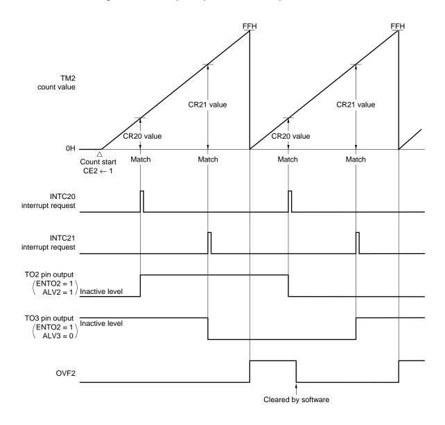
Figure 11-15. Compare Operation in 8-Bit Operation Mode
