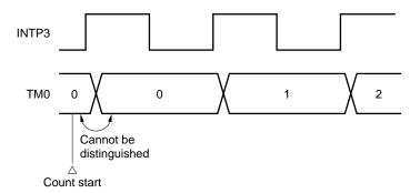
Figure 9-54. To Distinguish whether One or No Valid Edge has been Input with External Event Counter
