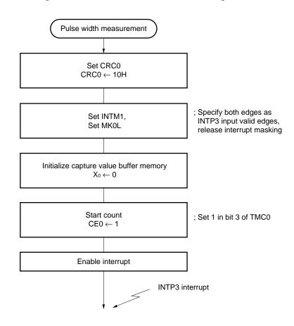
Figure 9-40. Interrupt Request Servicing that Calculates Pulse Width
