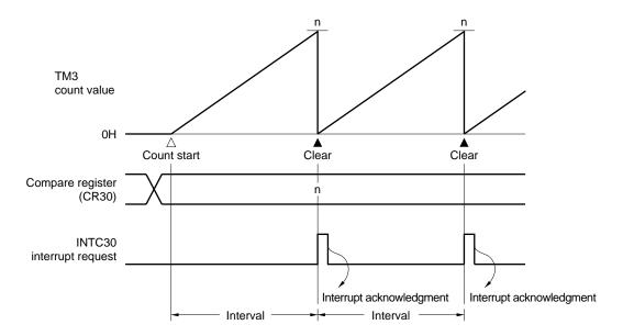
Figure 12-9. Interval Timer Operation Timing
