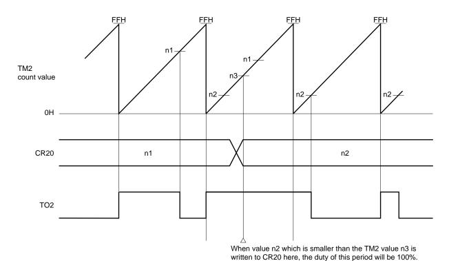
Figure 11-27. Example of 100% Duty with PWM Output
