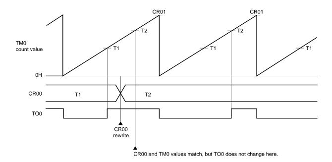
Figure 9-25. Example of Compare Register (CR00) Rewrite
