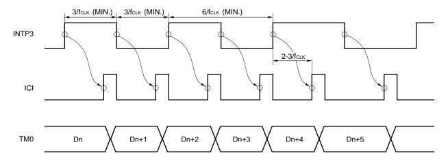
Remark ICI: INTP3 input signal after passing through edge detection circuit
