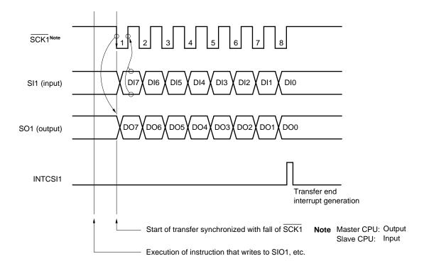
Figure 18-12. 3-Wire Serial I/O Mode Timing (2/2)
