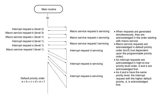
Figure 23-14. Examples of Servicing of Simultaneously Generated Interrupts
