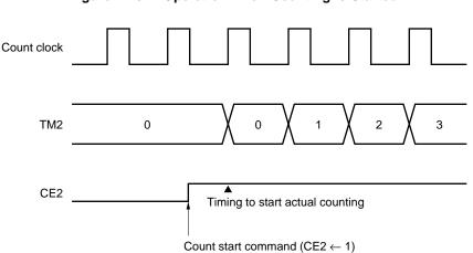
Figure 11-61. Operation when Counting is Started
