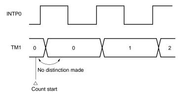
Figure 10-12. To distinguish whether One or No Valid Edge has been Input with External Event Counter
