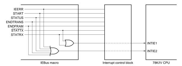
Figure 20-28. Configuration of Interrupt Control Block
