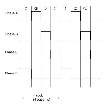
Figure 23-34. 1-2-Phase Excitation of 4-Phase Stepping Motor
