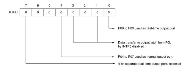
Figure 7-8. Real-Time Output Function Setting Procedure
