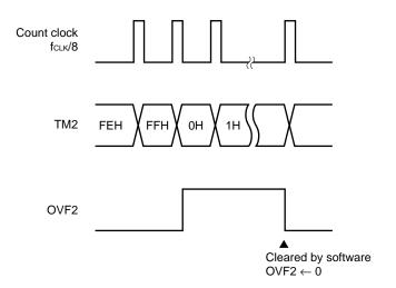
Figure 11-7. Basic Operation in 16-Bit Operation Mode (BW2 = 1)
