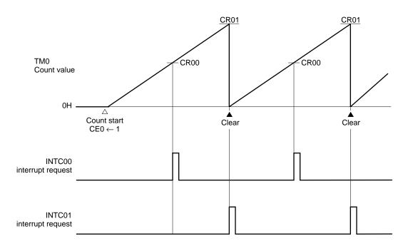
Figure 9-14. TM0 Clearance After Match Detection
