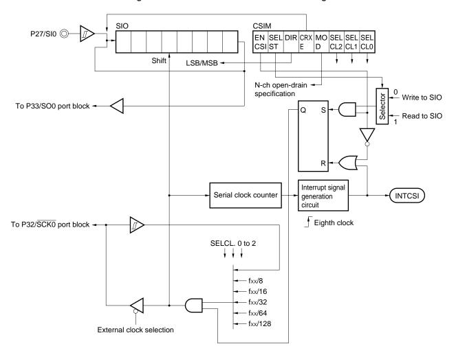
Figure 19-1. Clocked Serial Interface Block Diagram
