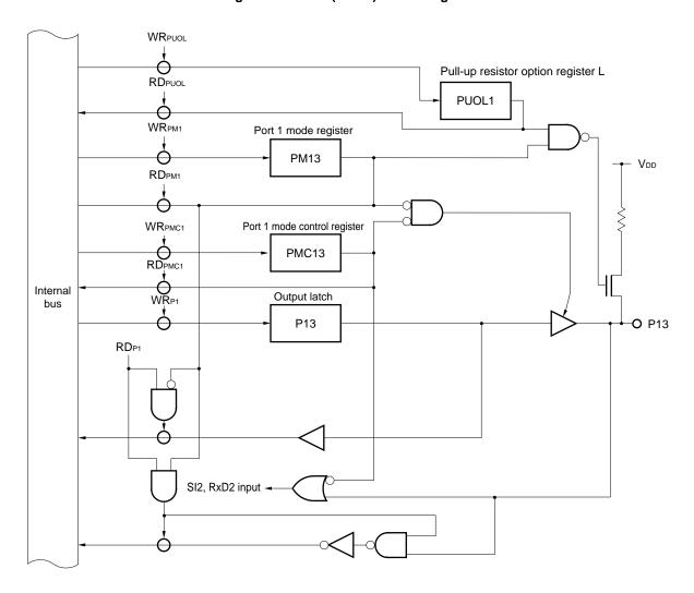
Figure 6-10. P13 (Port 1) Block Diagram
