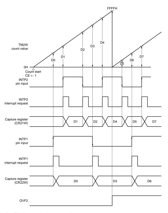
Figure 11-19. Capture Operation in 16-Bit Operation Mode
