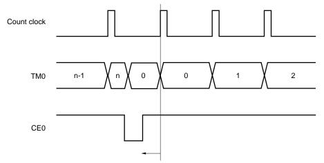
If the CE0 bit is set (to 1) before this count clock, the count starts from 0 on the count clock.
