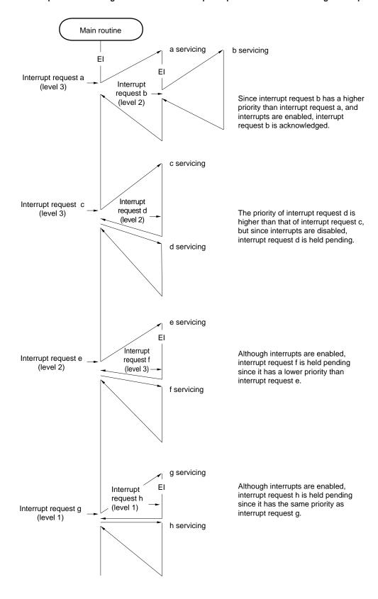
Figure 23-13. Examples of Servicing when Another Interrupt Request is Generated During Interrupt Service (2/3)
