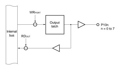
Figure 6-76. Port Specified as Output Port
