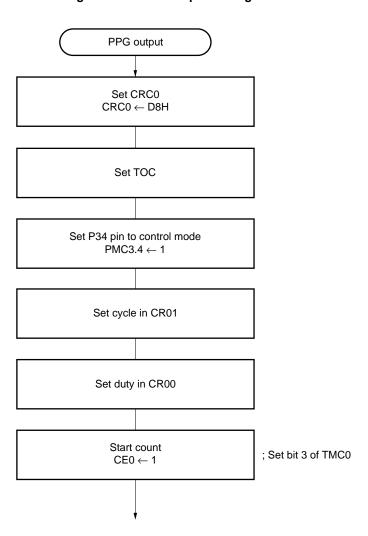
Figure 9-47. PPG Output Setting Procedure
