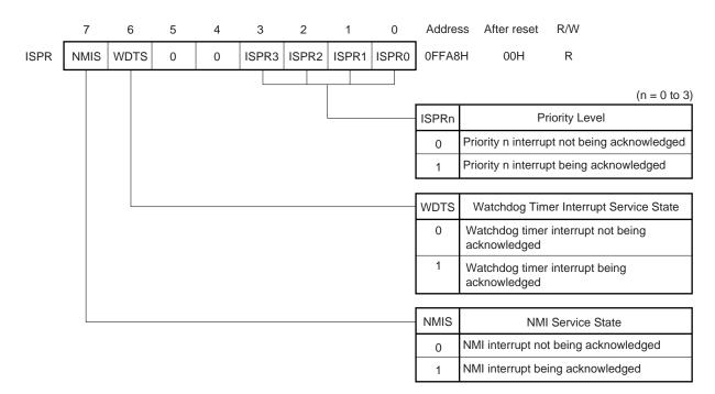
Figure 23-3. In-Service Priority Register (ISPR) Format
