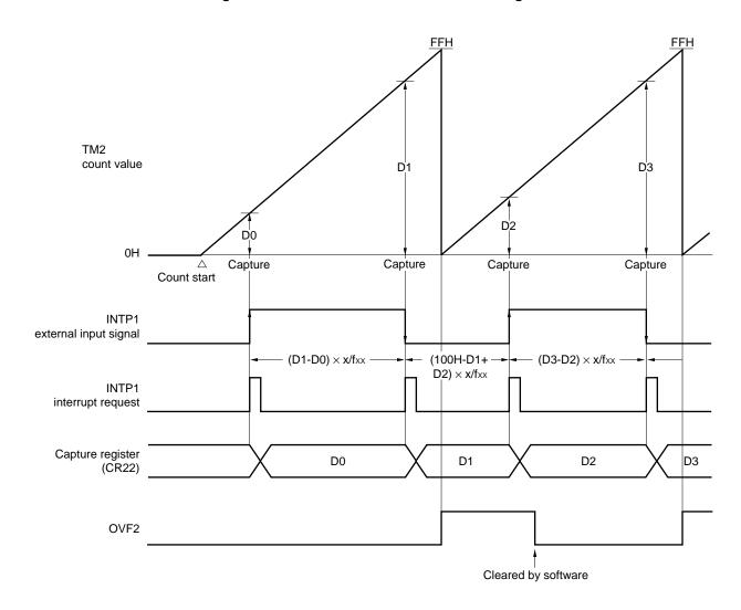
Figure 11-42. Pulse Width Measurement Timing
