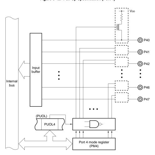
Figure 6-42. Pull-Up Specification (Port 4)
