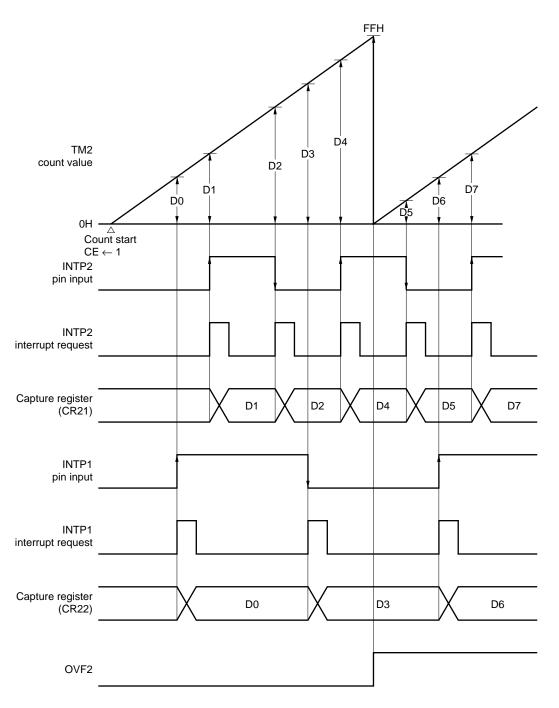
Figure 11-18. Capture Operation in 8-Bit Operation Mode
