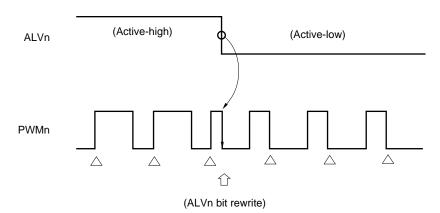
Figure 15-5. PWM Output Active Level Setting
