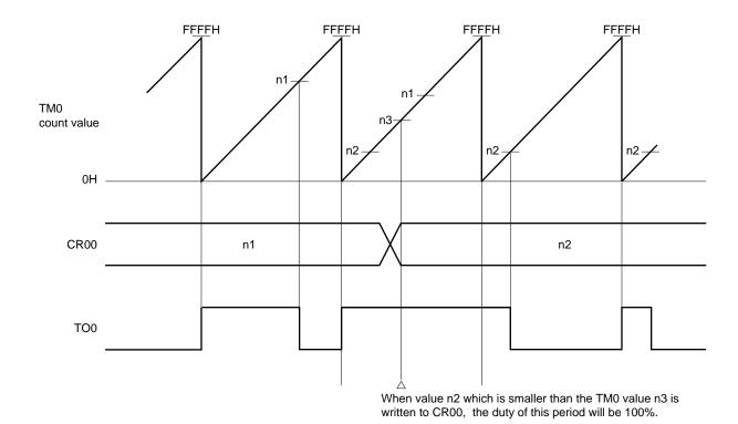
Figure 9-21. Example of 100% Duty with PWM Output
