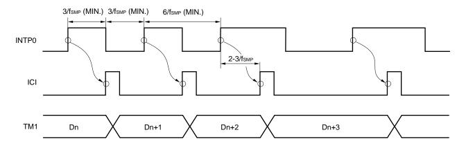
Remarks 1. ICI: INTP0 input signal after passing through edge detection circuit
