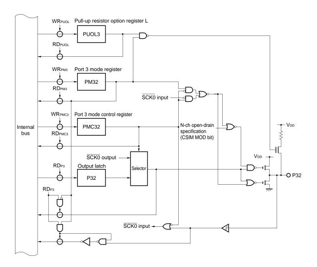
Figure 6-28. P32 (Port 3) Block Diagram
