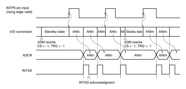
Figure 16-13. Hardware Start Select Mode A/D Conversion Operation
