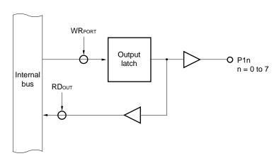
Figure 6-15. Port Specified as Output Port
