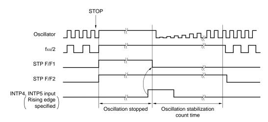
Figure 25-6. STOP Mode Release by INTP4/INTP5 Input
