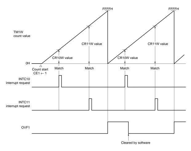
Figure 10-14. Compare Operation in 16-Bit Operation Mode
