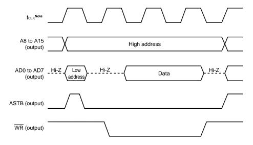
Figure 24-13. Access Wait Function Write Timing (2/2)
