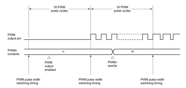
Figure 15-6. PWM Output Timing Example 1 (PWM pulse width rewrite cycle = 212/fpwmc)
