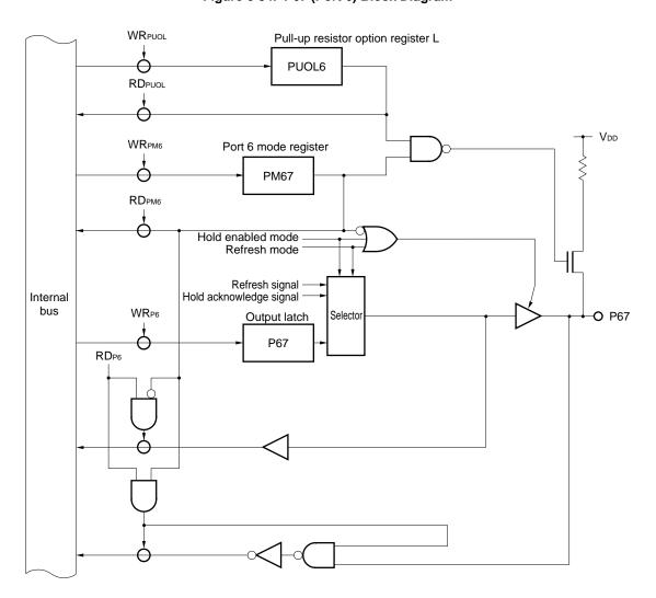
Figure 6-54. P67 (Port 6) Block Diagram
