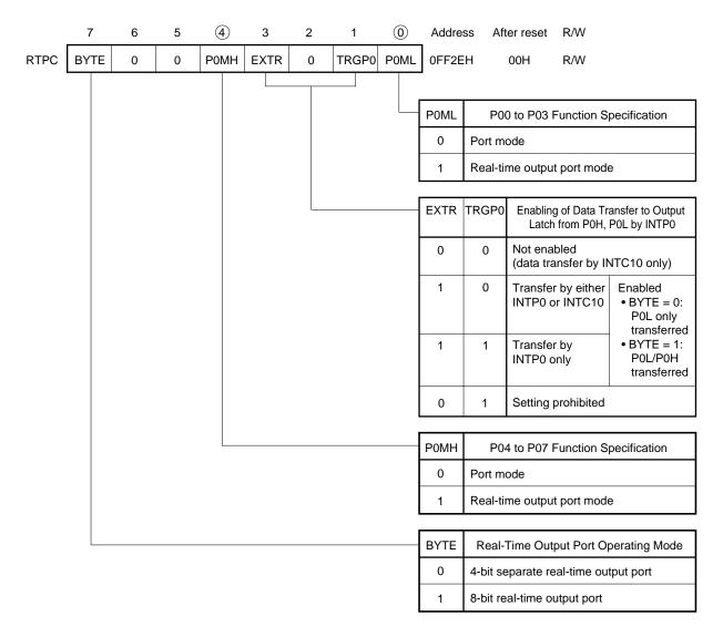
Caution When P0ML and P0MH bits are set (to 1), the corresponding port output buffer is turned on and the port 0 output latch contents are output irrespective of the contents of the port 0 mode register (PM0). The output latch contents should therefore be initialized before making a real-time output port specification.
