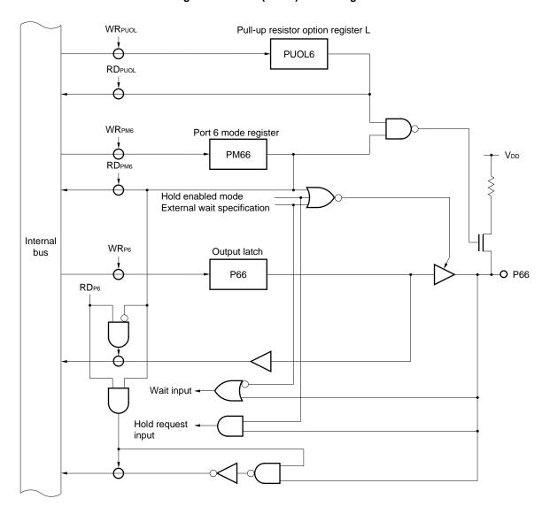
Figure 6-53. P66 (Port 6) Block Diagram
