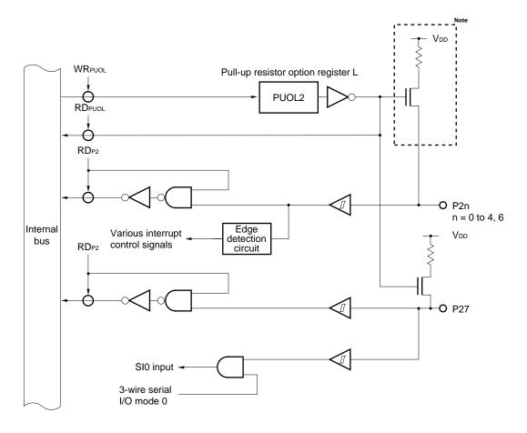
Note P20 and P21 do not have the circuitry enclosed by the broken lines.
