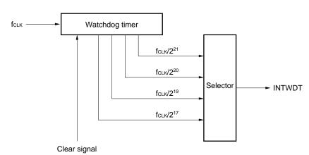
Figure 13-1. Watchdog Timer Block Diagram
