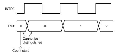
Figure 10-32. To Distinguish whether One or No Valid Edge has been Input with External Event Counter
