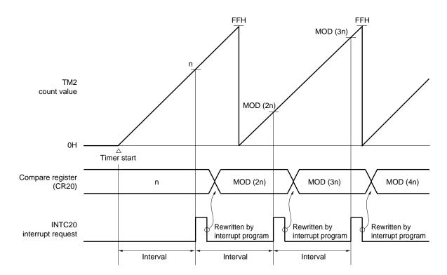
Figure 11-35. Interval Timer Operation (1) Timing
