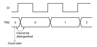
Figure 11-63. To Distinguish whether One or No Valid Edge has been Input with External Event Counter
