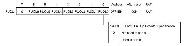
Remark When STOP mode is entered, setting PUOL to 00H is effective for reducing the current consumption.
