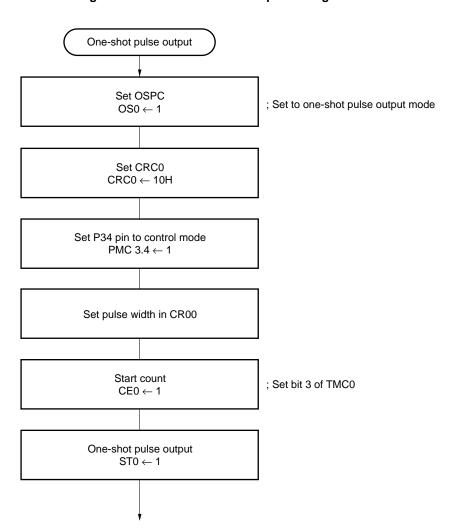
Figure 9-51. One-Shot Pulse Output Setting Procedure
