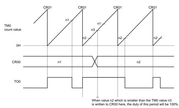
Figure 9-26. Example of 100% Duty with PPG Output
