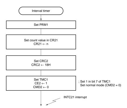
Figure 11-41. Interval Timer Operation (2) Setting Procedure
