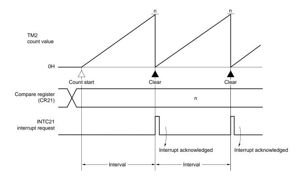
Figure 11-39. Interval Timer Operation (2) Timing
