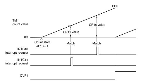
Figure 10-13. Compare Operation in 8-Bit Operation Mode
