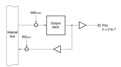
Figure 6-32. Port Specified as Output Port
