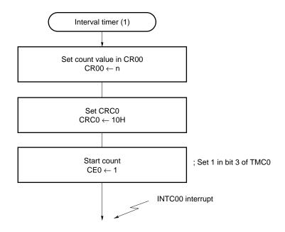
Figure 9-33. Interval Timer Operation (1) Interrupt Request Servicing
