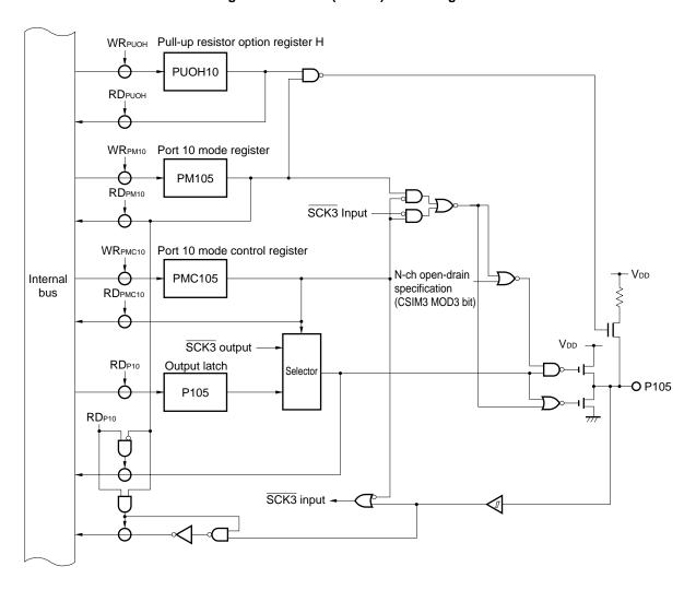
Figure 6-71. P105 (Port 10) Block Diagram
