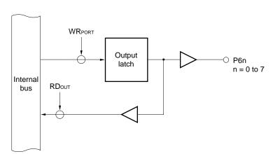
Figure 6-56. Port Specified as Output Port
