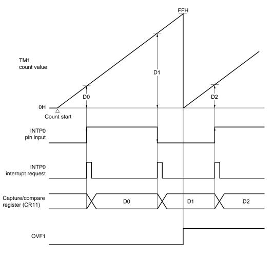
Figure 10-16. Capture Operation in 8-Bit Operation Mode
