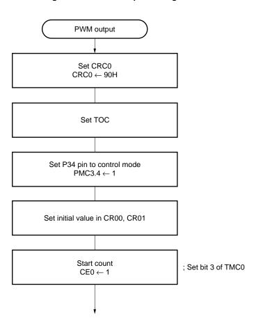
Figure 9-43. PWM Output Setting Procedure
