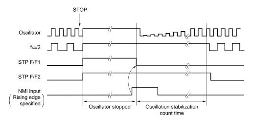
Figure 25-5. STOP Mode Release by NMI Input
