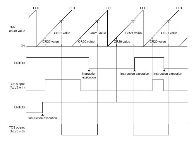
Figure 11-21. Toggle Output Operation
