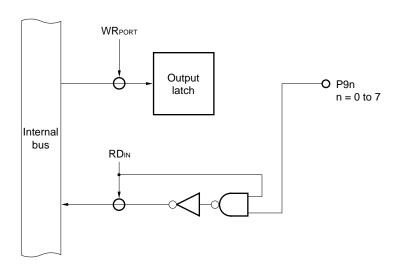
Figure 6-67. Port Specified as Input Port
