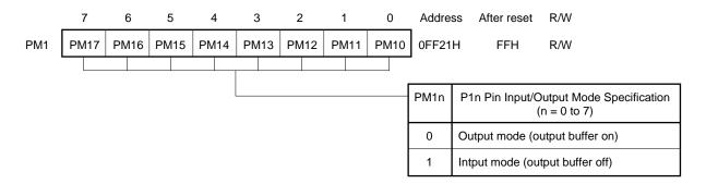
Figure 6-14. Port 1 Mode Control Register (PMC1) Format
