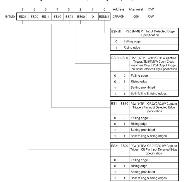
Figure 22-1. External Interrupt Mode Register 0 (INTM0) Format
