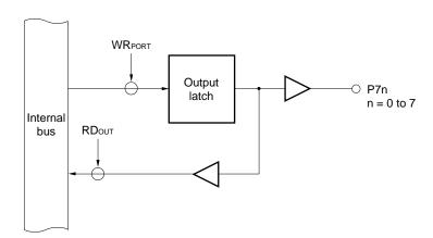
Figure 6-62. Port Specified as Output Port
