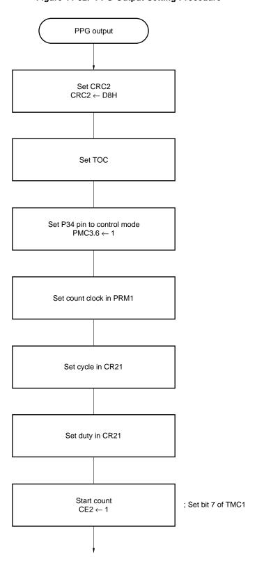
Figure 11-52. PPG Output Setting Procedure
