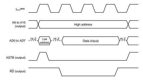
Figure 24-12. Access Wait Function Read Timing (2/2)
