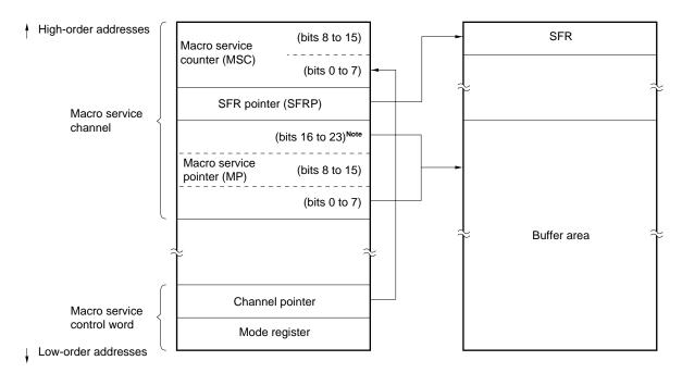
Figure 23-26. Type B Macro Service Channel
