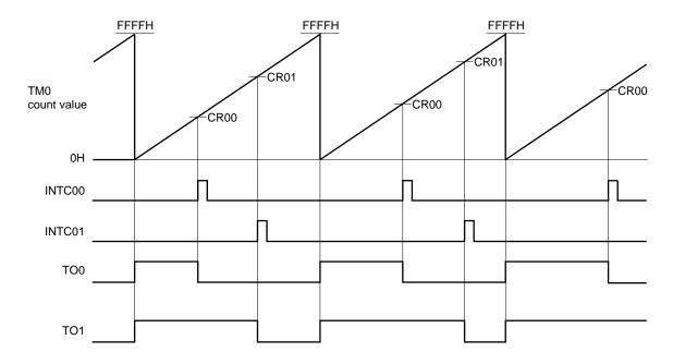
Figure 9-18. Example of PWM Output Using TM0
