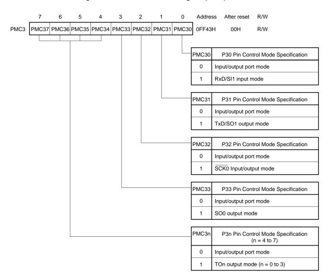
Figure 6-31. Port 3 Mode Control Register (PMC3) Format
