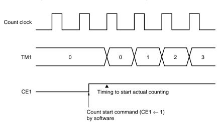
Figure 10-30. Operation when Counting is Started
