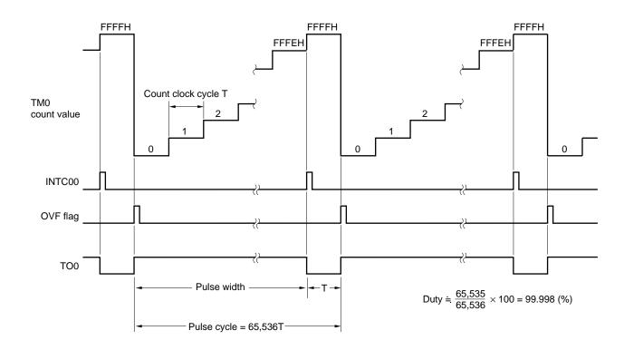
Figure 9-19. Example of PWM Output when CR00 = FFFFH
