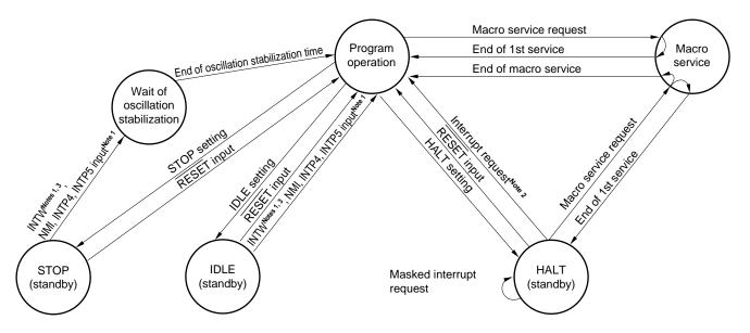
Figure 25-1. Standby Mode Transition Diagram
