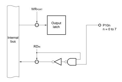
Figure 6-77. Port Specified as Input Port
