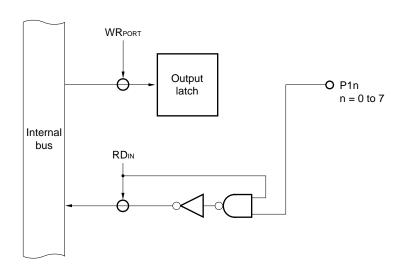
Figure 6-16. Port Specified as Input Port
