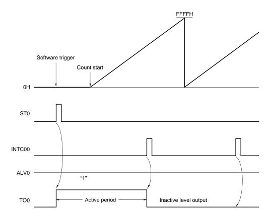
Figure 9-29. Example of Software Triggered One-Shot Pulse Output
