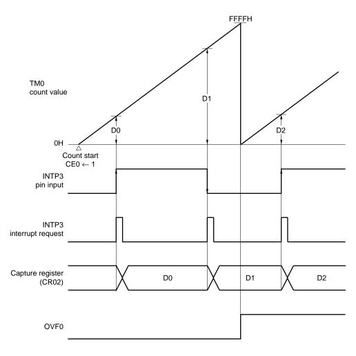
Figure 9-15. Capture Operation
