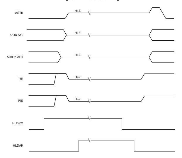
Figure 24-21. Hold Mode Timing
