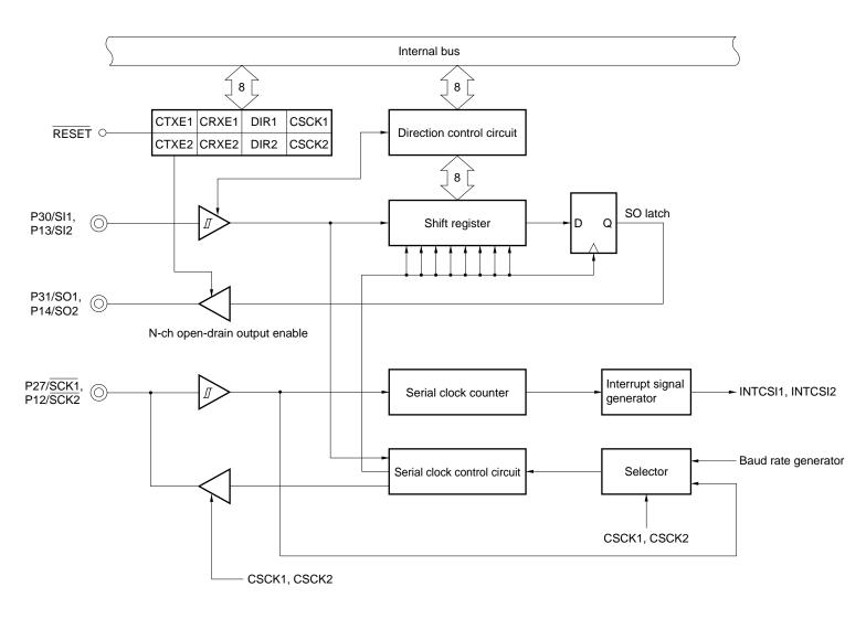
Figure 18-10. 3-Wire Serial I/O Mode Block Diagram
