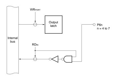
Figure 6-57. Port Specified as Input Port
