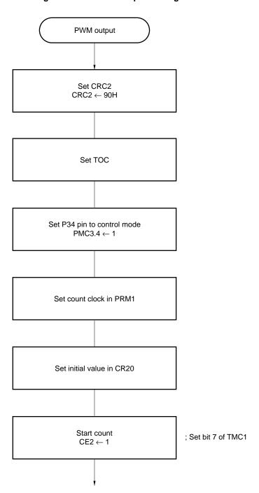
Figure 11-48. PWM Output Setting Procedure
