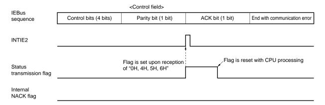
Figure 20-17. Interrupt Generation Timing (in case of <2>, <5>)
