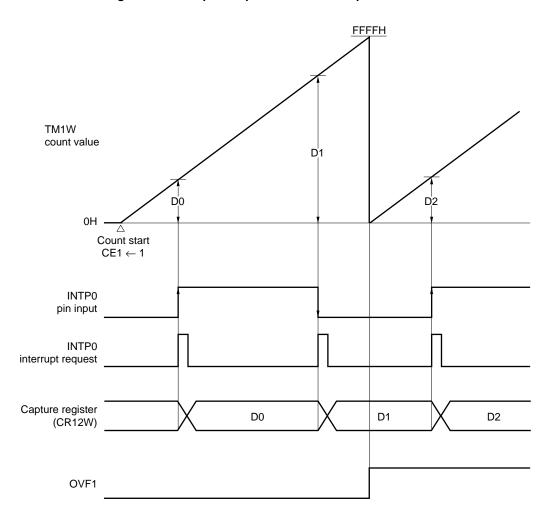
Figure 10-17. Capture Operation in 16-Bit Operation Mode
