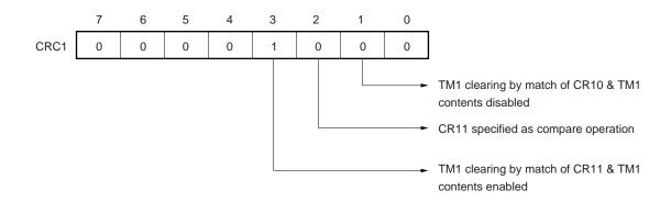
Figure 10-25. Interval Timer Operation (2) Setting Procedure
