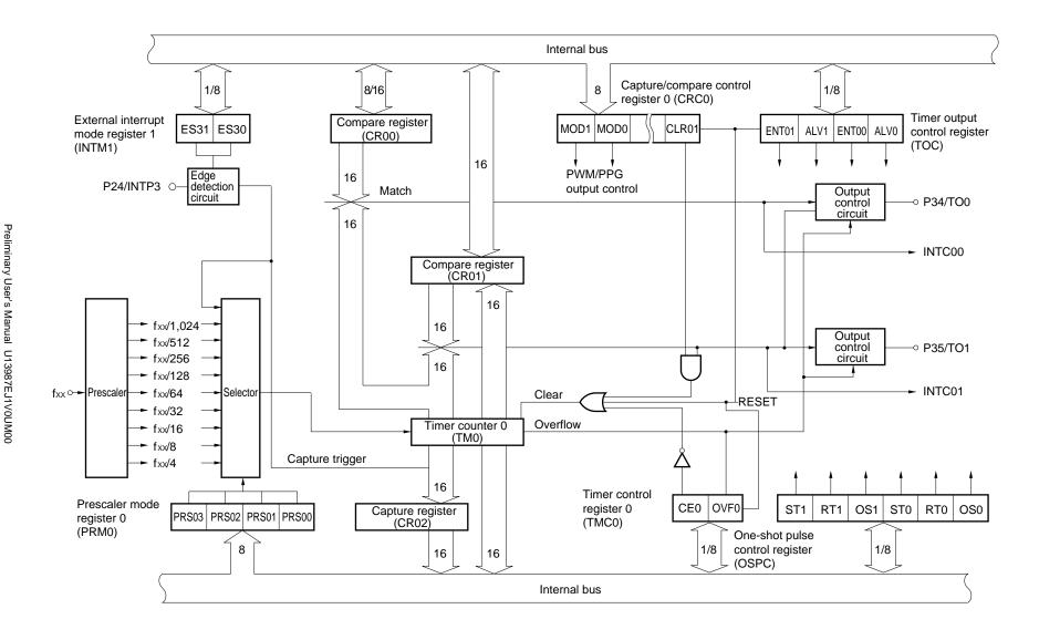
Figure 9-1. Timer/Event Counter 0 Block Diagram
