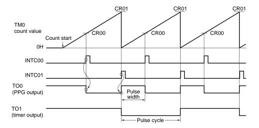
Figure 9-23. Example of PPG Output Using TM0
