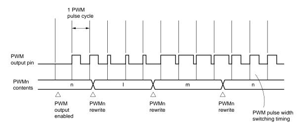
Figure 15-7. PWM Output Timing Example 2 (PWM pulse width rewrite cycle = 28/fpwmc)
