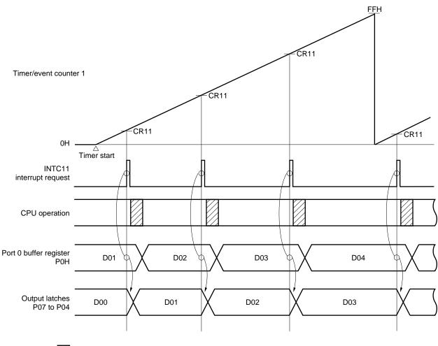
Figure 7-4. Real-Time Output Port Operation Timing
