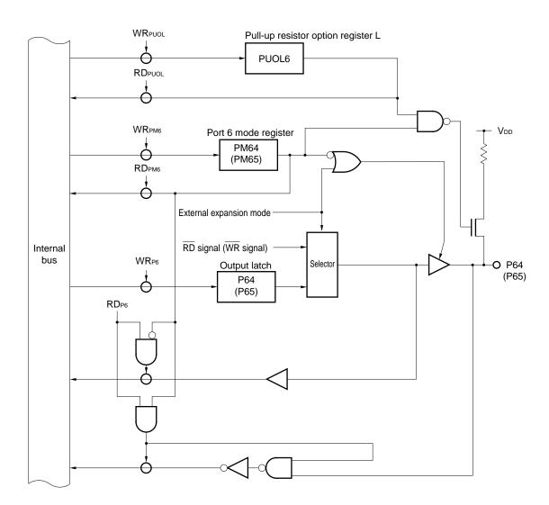
Figure 6-52. P64 and P65 (Port 6) Block Diagram
