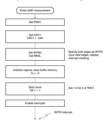
Figure 10-28. Pulse Width Measurement Setting Procedure
