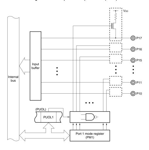
Figure 6-19. Pull-Up Resistor Specification (Port 1)
