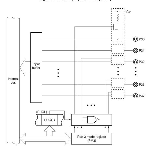
Figure 6-36. Pull-Up Specification (Port 3)
